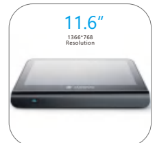
11.6" 1366*768 Resolution Projective Capacitive Touch Screen
